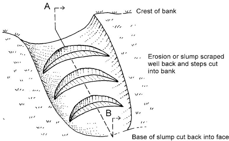
Figure 29. A suggested procedure for restoration of minor breaks or slumps in earthwork banks; successive details of the cross-section A-B are shown below.
