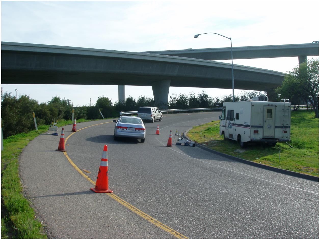
Figure 11. The Fresno monitoring site showing the monitoring vehicle and the remote sensing detectors and speed and acceleration bars.
