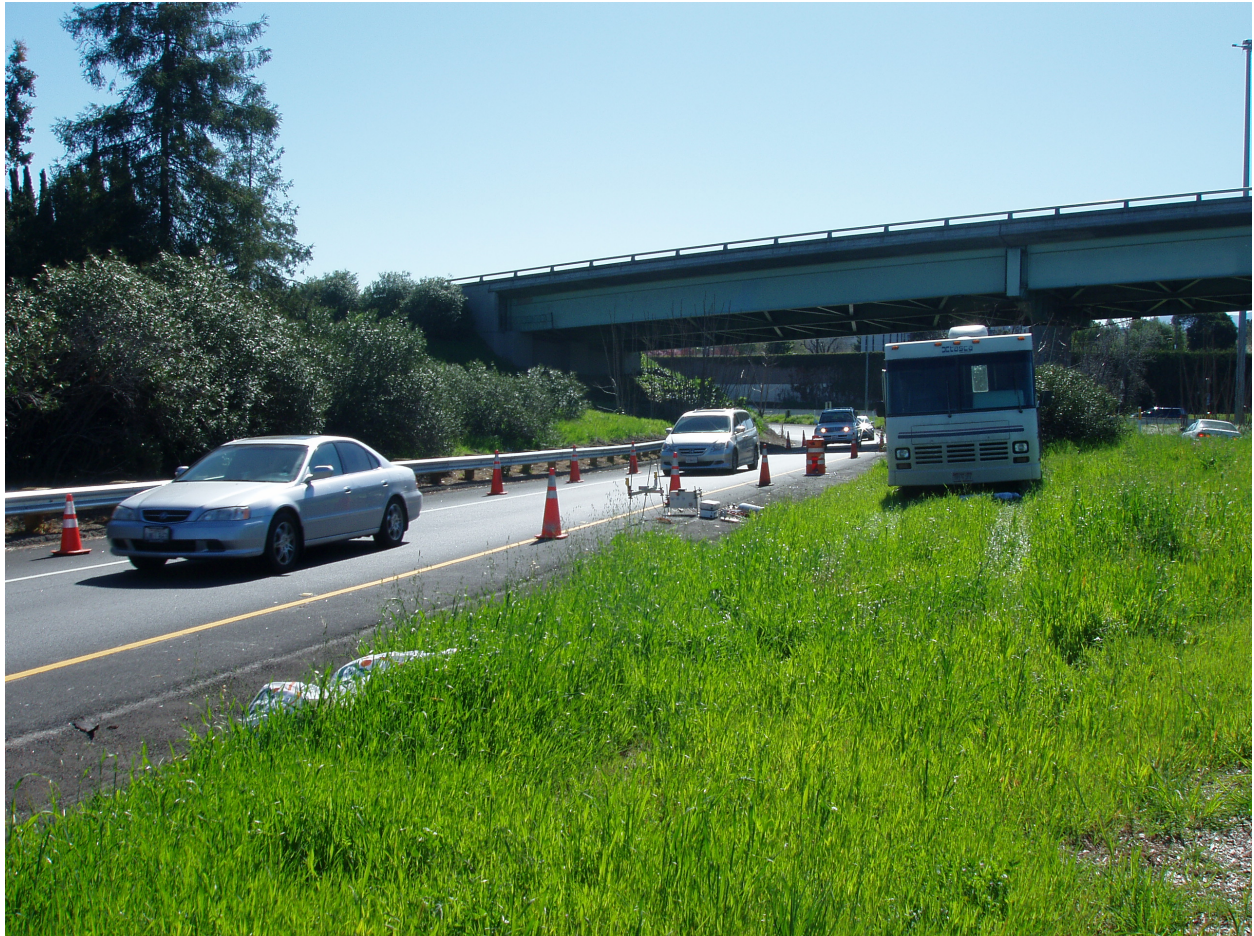
Figure 2. The San Jose monitoring site showing the monitoring vehicle and the remote sensing detectors and speed and acceleration bars on the near side of the roadway.
