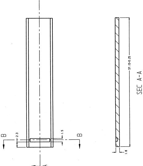
Figure B3. Machine drawing of filter shutter.
