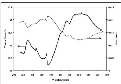
Figure 5. Baseline transmittance and absorbance spectra for a commercial double-beam spectrophotometer with automatic baseline correction.
