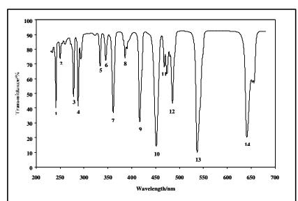
Figure 4. The transmittance spectrum of SRM 2034 holmium oxide solution wavelength standard with the certified bands indicated.
