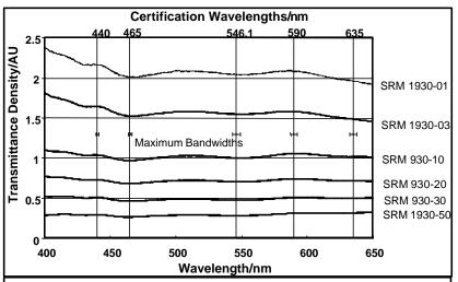
Figure 2. Transmittance density spectra for SRMs 930 and 1930 illustrating the wavelengths of certification and maximum bandwidths for use.
