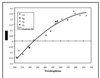
Figure 3. Wavelength calibration of the ACD reference spectrophotometer using atomic pen lamps.
