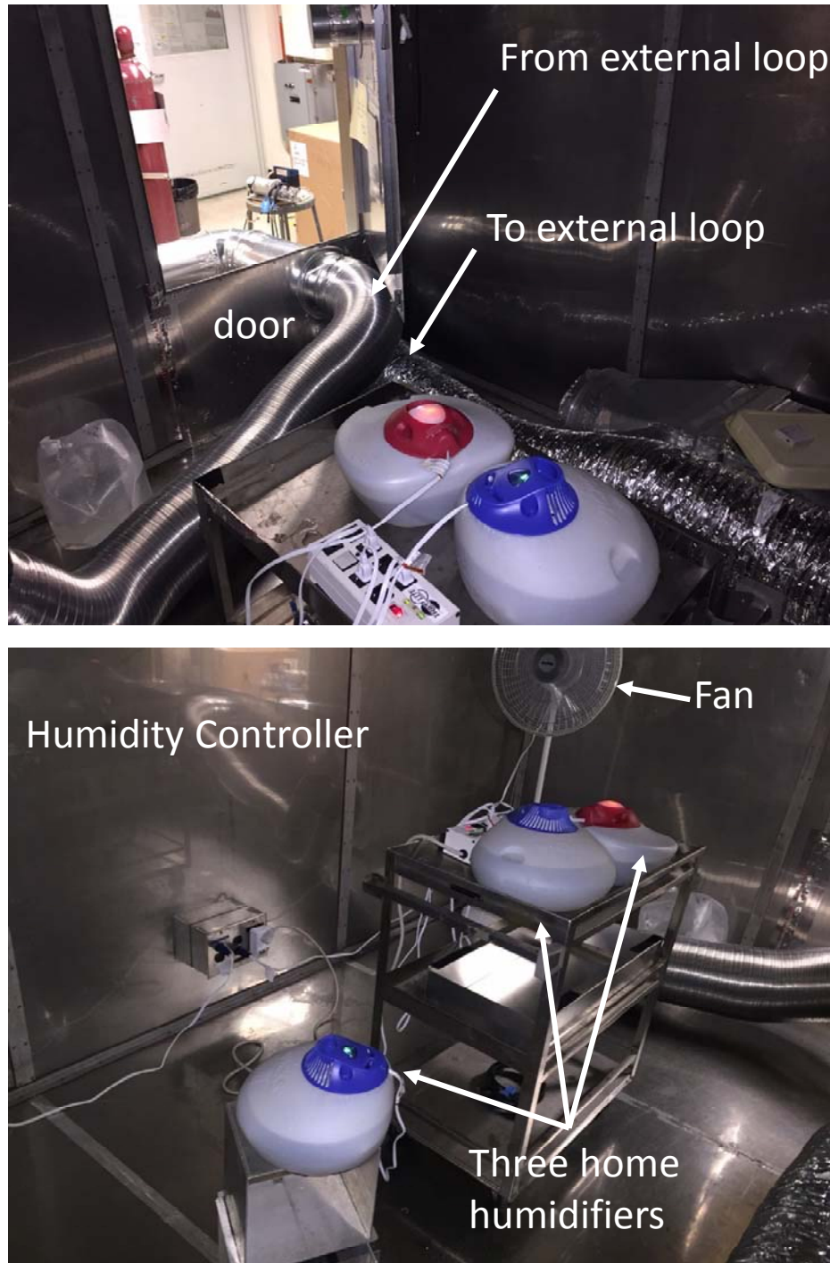
Figure 4.1.3. Interior of room-sized chamber
