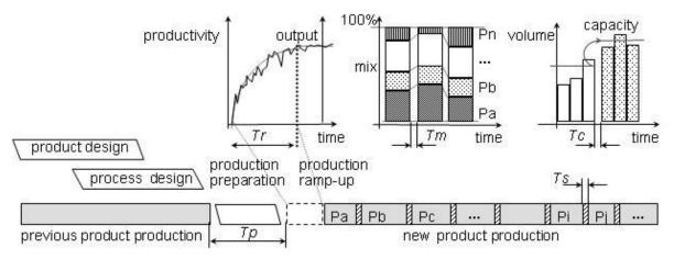
Figure 1. Production system under dynamic conditions.
