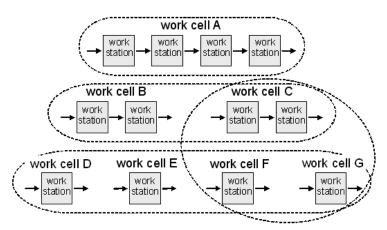
Figure 8. Set of different work cells.
