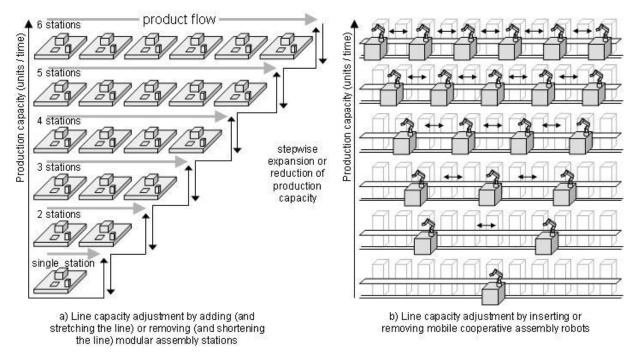
Figure 9. Development of advanced manufacturing technologies to enhance reconfigurability supporting abilities in manufacturing firms
