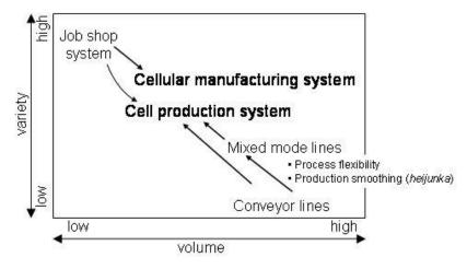
Figure 2. Trajectories towards cellular manufacturing and cell production system
