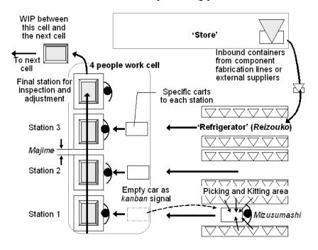
Figure 7. The pulling of materials flow in the cell production system
