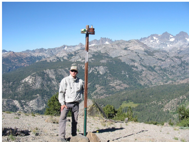
Figure 4. Ozone Passive Sampler Mounted on a Wooden Stand 2-m Aboveground – Fish Creek site on the San Joaquin River Drainage.
